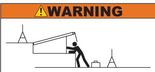
Always post safety warnings and barricade the work area at dock level and ground level to prevent unauthorized use of the equipment before maintenance is complete.
