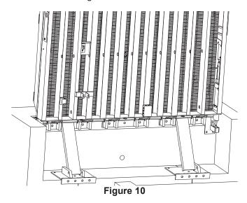
13. Insert the hinge pins. Start from the center and work outwards.
