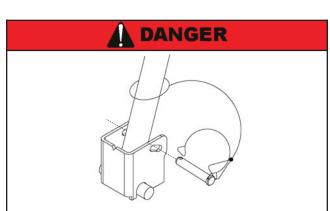
A maintenance prop permanently attached and hinged to the unit with means for lock out/tag out requirements (per OSHA 1910.147) is included with each pit style dock leveler. In addition, it is recommended and good safety practice to use an additional means to support the dock platform and lip anytime when physically working in front of or under the dock leveler. This additional means may include, but not limited to a boom truck, fork truck, stabilizing bar or equivalent.
