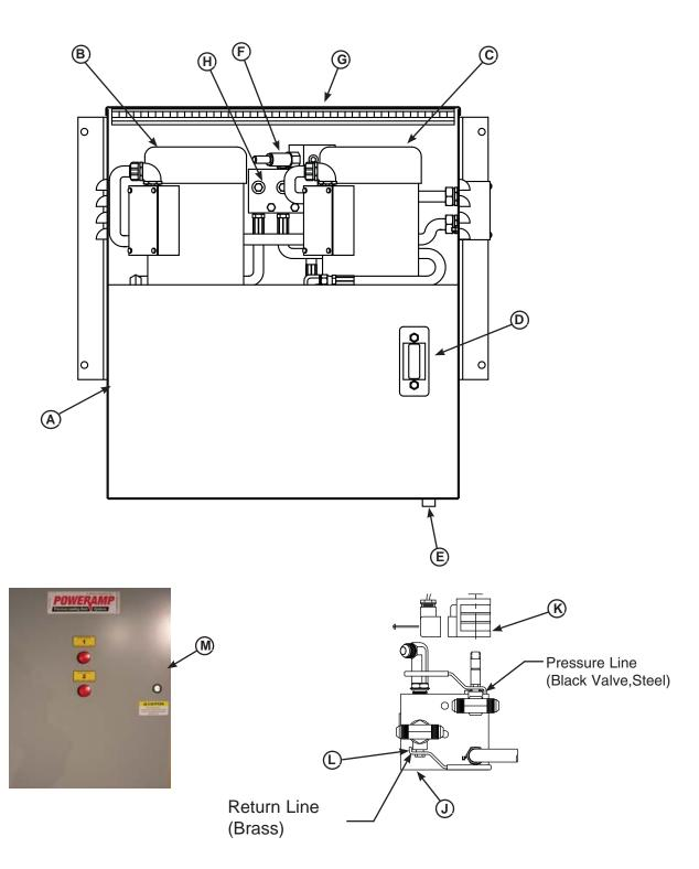
A — Pump Station B — Pump Motor #1 C — Pump Motor #2
