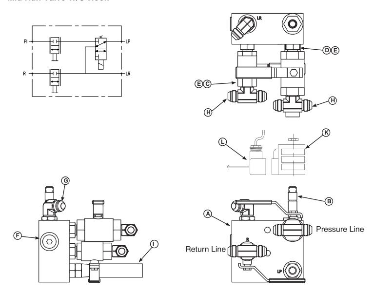
Coil De-Energized when lever or restraint is Engaged **not** in use. Coil Energized when lever or restraint is Engaged.
