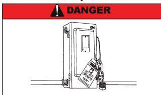
Hydraulic and electrical power must be OFF when servicing the equipment. For maximum protection, use an OSHA approved locking device to lock out all power sources. Only the person servicing the equipment should have the key to unlock the device.
