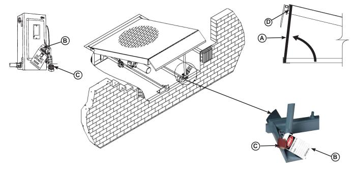
A— Maintenance Prop B—Tag Out Device C—Lock Out Device D—Front Header
