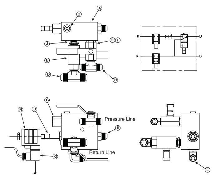
Coil De-Energized when lever or restraint is Engaged **not** in use. Coil Energized when lever or restraint is Engaged.
