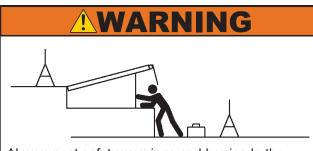
Always post safety warnings and barricade the work area at dock level and ground level to prevent unauthorized use of the unit before maintenance is complete. When working with electrical or electronic controls, make sure that the power source has been tagged (A) and locked out (B) according to OSHA regulations and approved local electrical codes (see Figure 21).
