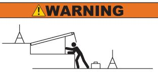
Always post safety warnings and barricade the work area at dock level and ground level to prevent unauthorized use of the unit before maintenance is complete.
