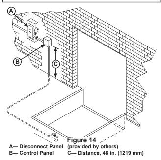
1. Mount the push-button control panel (**B**) so bottom of control panel-to-dock floor distance (**C**) is approximately 48 in. (1219 mm). See Figure 14.
