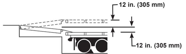
The DM mechanical dock leveler is designed to compensate for a maximum  $\pm 12$  in.\* (305 mm) of height difference between the loading dock and the transport vehicle's bed. DO NOT use the dock leveler if the transport vehicle's bed is more than 12 in. (305 mm) higher or lower than the dock floor.
