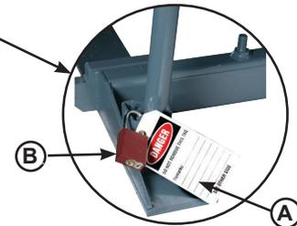
A— Tag Out Device    B—Lock Out Device    C— Maintenance Prop    D— Header
