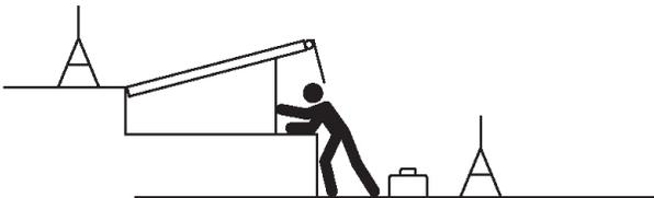
Always post safety warnings and barricade the work area at dock level and ground level to prevent unauthorized use of the unit before maintenance is complete.
