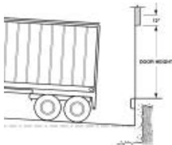
D. Check the heights of incoming carriers that will be utilized at this door, to ensure that the head pad is of proper elevation to accommodate the height range of these vehicles.
