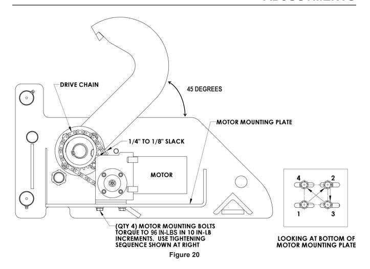
LUBRICATE DRIVE CHAIN AND LIMIT SWITCH MOUNTING BRACKET. USE
