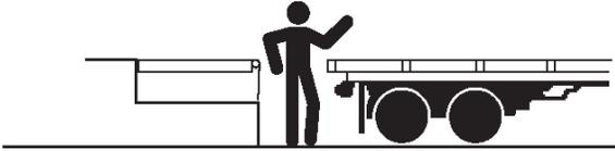
Stay clear of dock leveling device when the transport vehicle is entering or leaving area.
